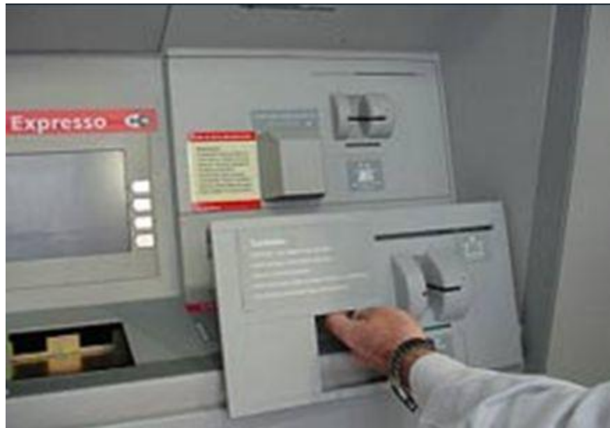
Figure 3: An ATM skimmer panel that fits directly on top of the real ATM (Krebs, 2010).
