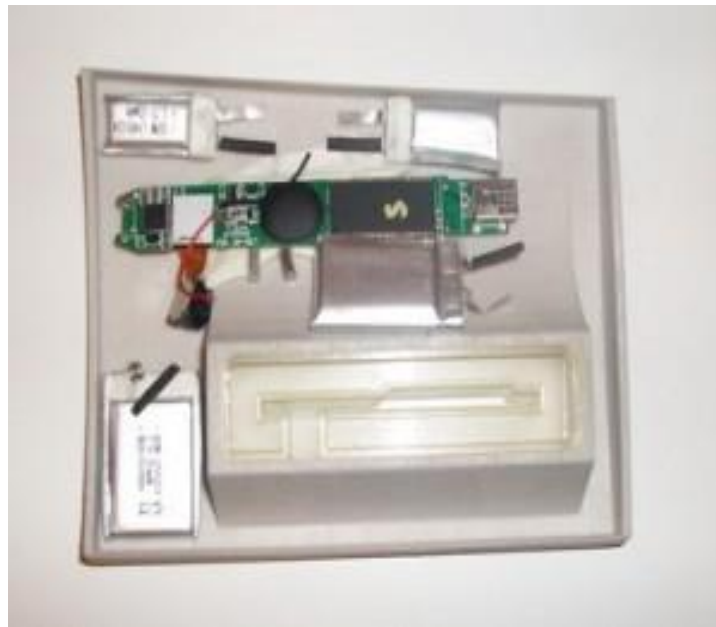
Figure 5: Audio skimmer for Diebold ATMs identified by five European nations (Krebs, 2010).
