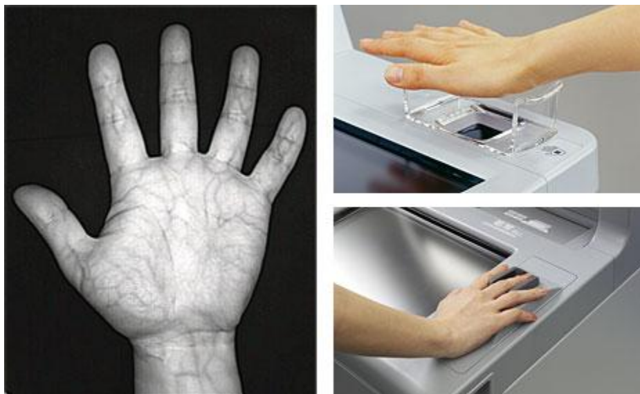
Figure 1: Fujitsu image of veins through a palm image (Left), Fujitsu palm vein reader (Top Right), Hitachi finer vein reader (Bottom Right) (Strickland, 2012).
