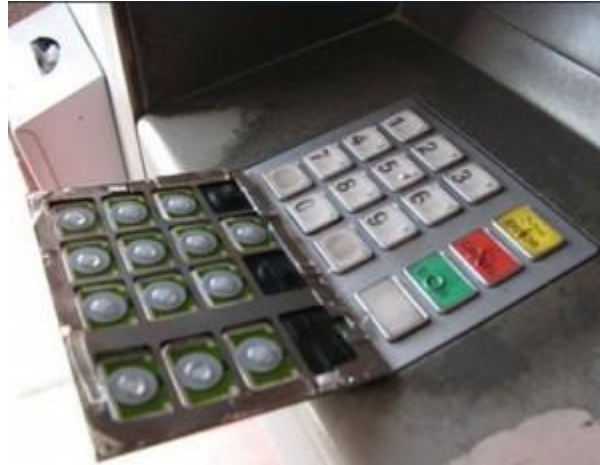
Figure 4: ATM PIN capture overlay device pulled back to reveal the legitimate PIN entry pad (Krebs, 2010).
